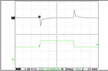
Figure 5: Output voltage response to step-change in load current (50 % -75 % -50 % of Iout(max); dI/dt = 0.1 A/ $\mu$ s). Load cap: 15  $\mu$ F tantalum cap and 1  $\mu$ F ceramic cap. Ch 1: Vout (1 V/div), Ch 2: Iout (5 A/div).
